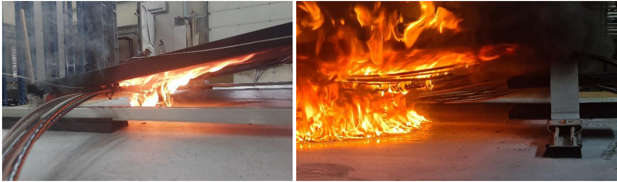
Figure 16 Detection cables on fire 1 min (left) and 6 min (right) after the ignition (FotoPortal (left 050522d-001, right 050522d-002))
