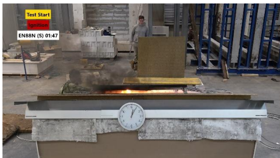
Figure 25 Delamination of solar cells and flame propagation over the top of the PV panel (FotoPortal 050522d-059)
