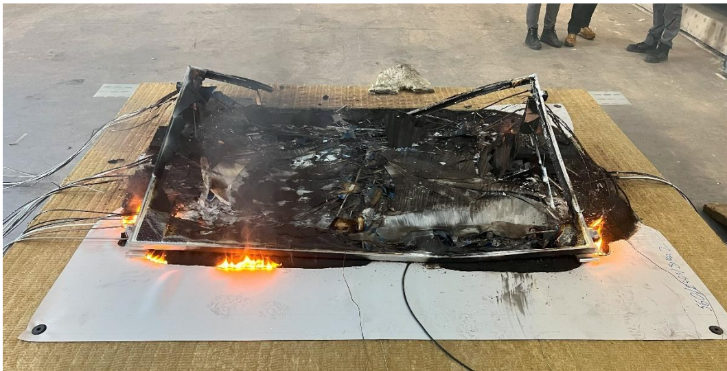
Figure 21 Shattered PV panel and flame residues on the roofing membrane (FotoPortal 050522d-031)
