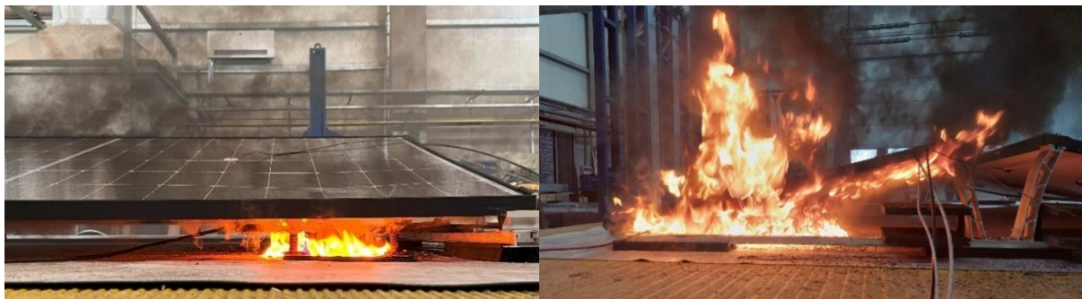
Figure 28 Flame spread over LHD system after 5-6 min: front (left) and side (right) view (FotoPortal (left 050522d-084, right 050522d-085))
