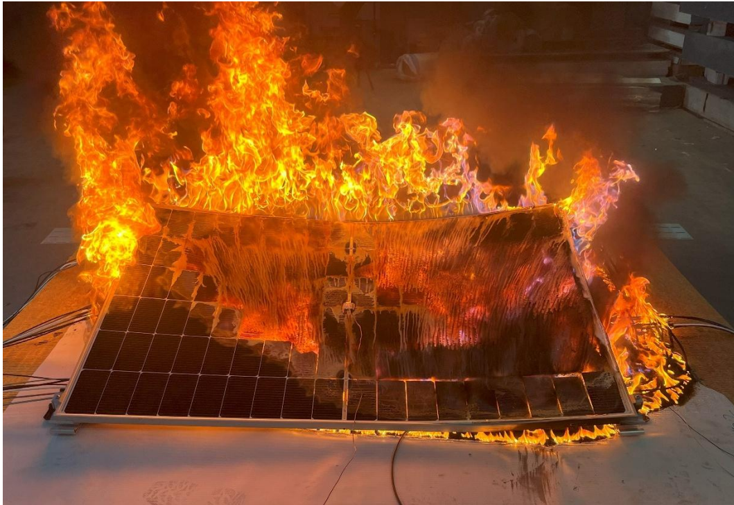
Figure 20 PV module engulfed in flame, along with blue flames coming from the cables (top right corner) (FotoPortal 050522d-030)
