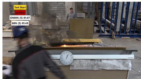
Figure 25 Delamination of solar cells and flame propagation over the top of the PV panel (FotoPortal 050522d-059)
