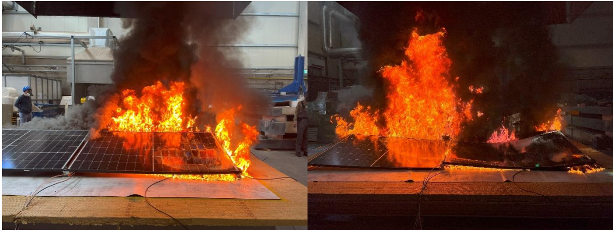
Figure 29 Flame spread over the first PV module (left) and towards the third and fourth modules (right), 8 minutes after ignition (FotoPortal (left 050522d-086, right 050522d-087))
