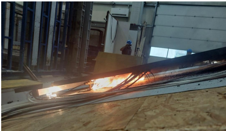
Figure 24 The extent of fire on the specimen just after stopping arc generation at 2 min (FotoPortal 050522d-058)
