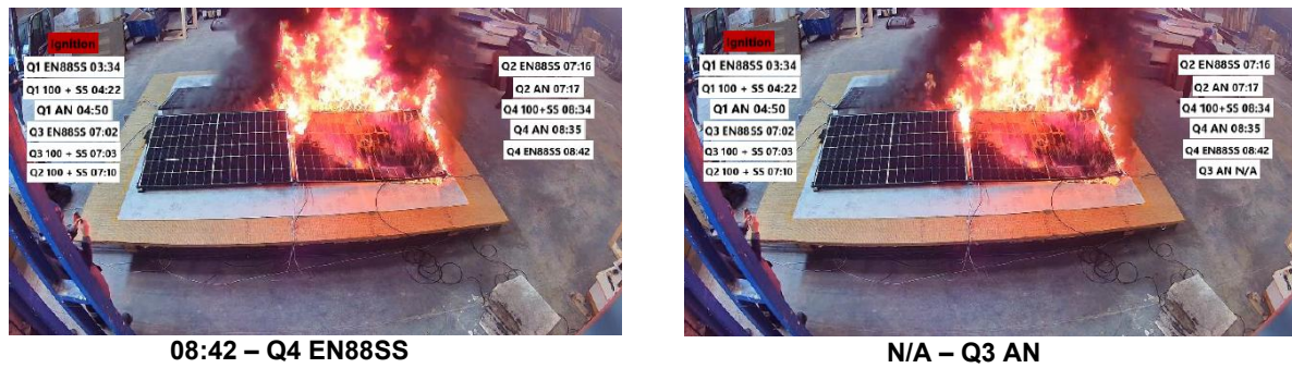
Figure 34 Aerial camera snapshots of LHD-4 during alarm activation (white boxes show the type of LHD cables and their detection times). Times are given in min:s. (FotoPortal from 050522d-138 to 050522d-149)
