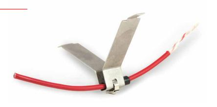
Beam clips may be used to support linear heat detection cable directly (in this case a separate silicone sleeve is required) or fixed to other mounting brackets and used to affix the bracket to a RSJ/I-beam or equivalent.
